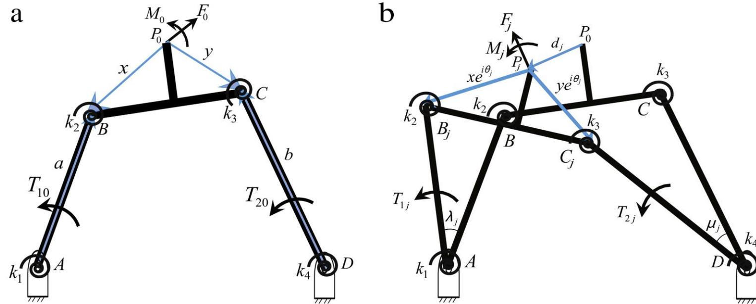
Fig. 2. A schematic view of a pseudo-rigid-body four-bar and its displaced configuration with the vector definitions.
