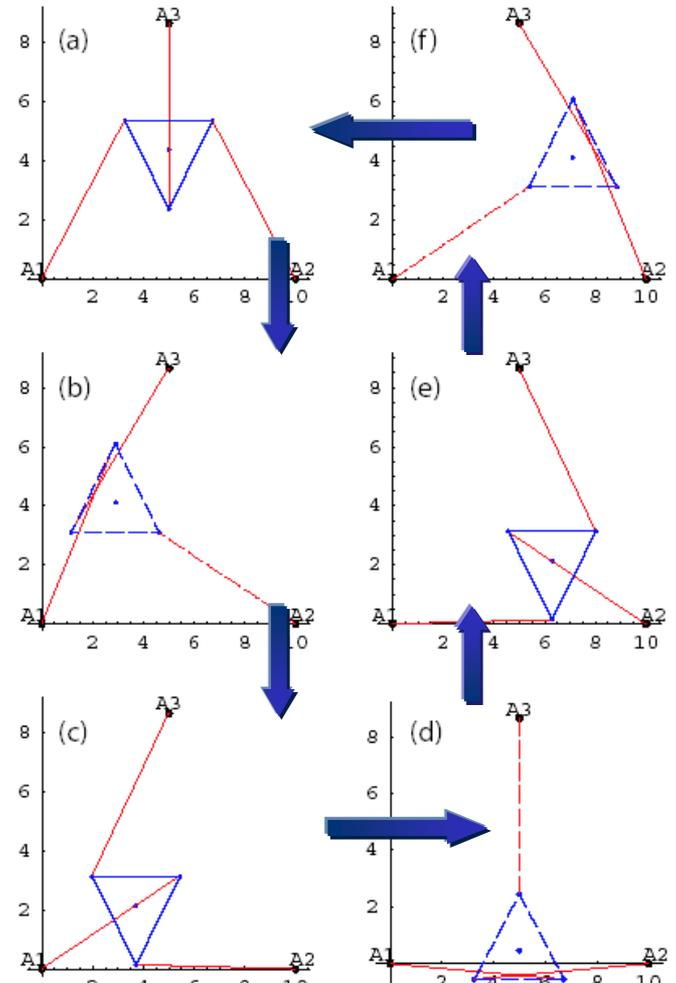
A tri-stable compliant mechanism
