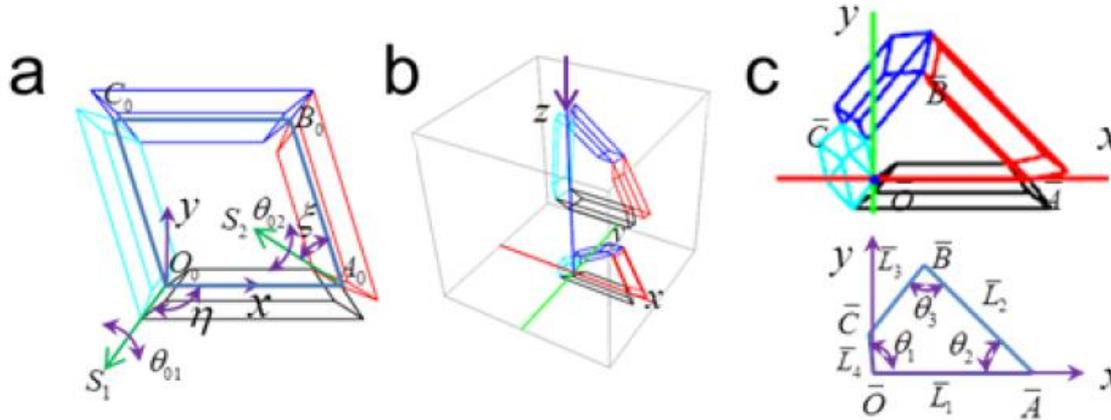
Table 5.14: Initial, rotated, projected and measured points that define the structure of DNA origami Bennett linkage
