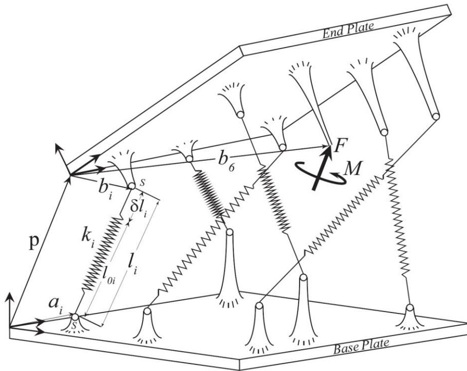
Fig. 1. A schematic view of a general compliant Stewart-Gough platform.
