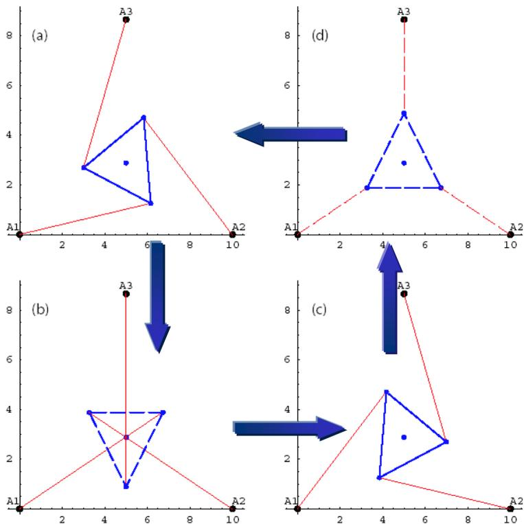
A bi-stable compliant mechanism
