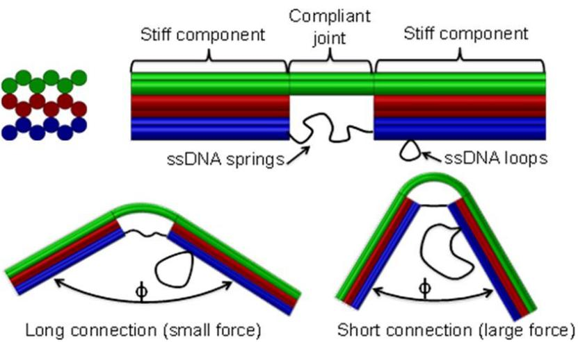
A design of compliant DNA joint
