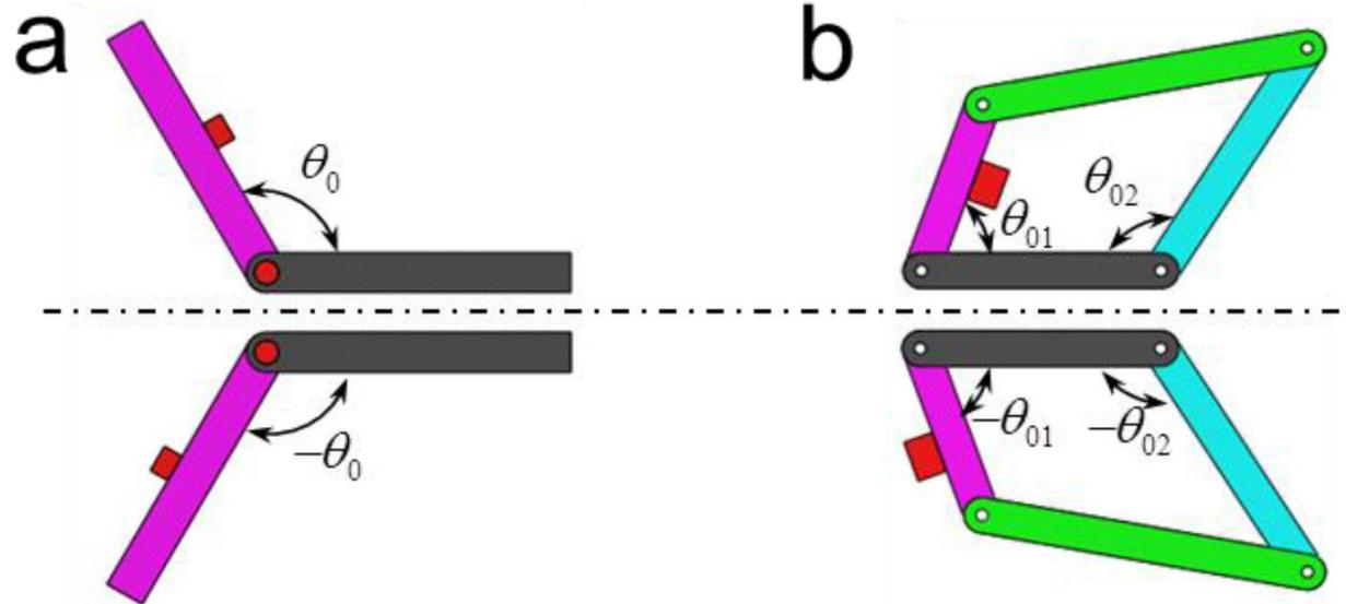
Symmetrical (mirrored) configurations distinguished by a designed feature (red box on the purple link). (a) Positive and negative revolute joint angles. (b) Symmetrical configurations of planer four-bar linkage.
