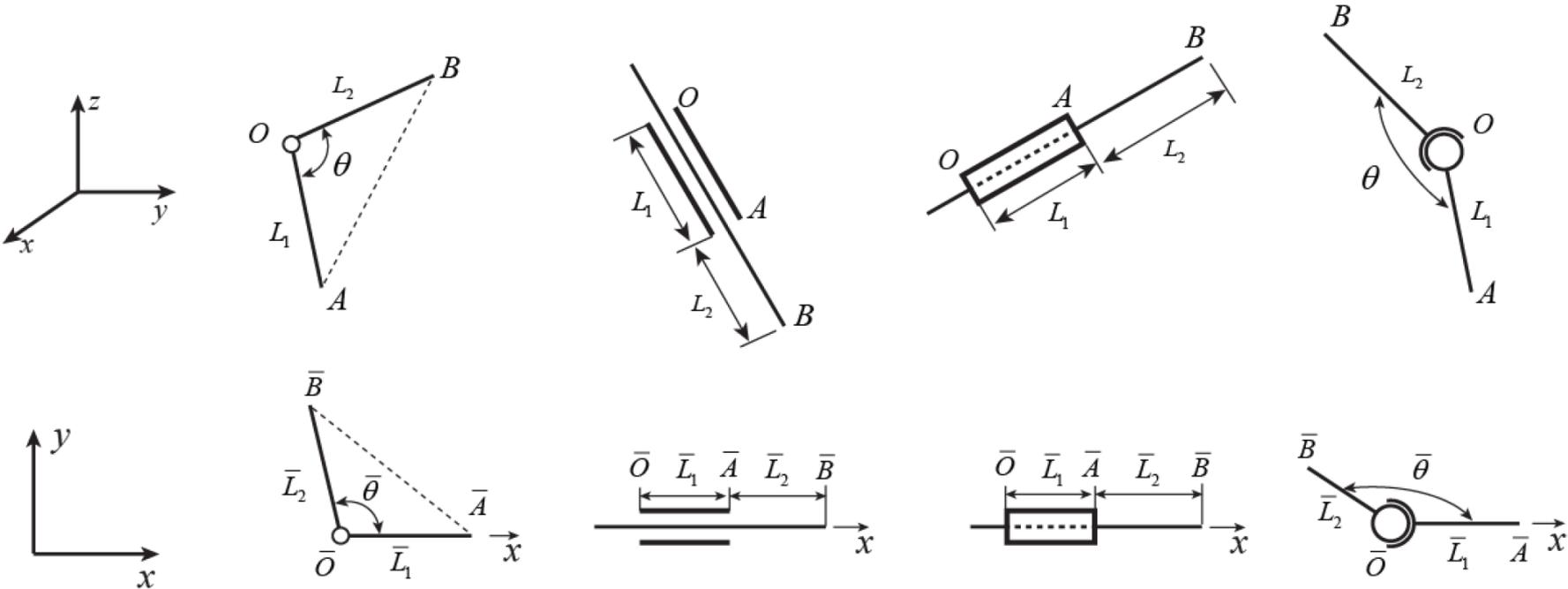
**Fig. 1.** Kinematic parameters of revolute, prismatic, cylindrical and spherical joints (from left to right) are 3D (top) in nature. They are projected to a  $x$ - $y$  plane (bottom).
